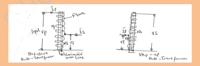
The auto-transformer is less expensive than the double-wound transformer but its use is limited because of the danger inherent in the direct electrical connections which exist between the input and output terminals. Auto-transformers are often employed in Ac motor-starters to reduce the pressure applied to the motor during the starting period.
