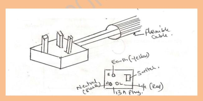
(c) The flexible cables are usually three in a cord of wire which is marked with the following colours, Red; black and Yellow. It is of different diameters but this very one is of 1.5mm<sup>2</sup> each. This is connected to a 13A plug that has three terminals.
