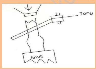
1. Upsetting is a forging operation in which the cross sectional area of the material (work piece) is increased at the expense of the length.
