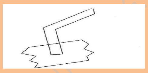
3. Bending: bending a straight rod in a hardy hole
