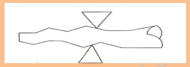
2. Drawing down is a forging operation in which the length of the material (work piece) is increased at the expense of the cross-sectional area.
