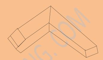
Used in corners of frame or carcasses where member meet at right angles.
