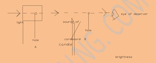
A small hole is punched in each of the cardboards A and b. They are placed in a straight line together with a light source. An observer is situated on the other side B. it will be found that the observer can only see light if the cardboards are well aligned. Light will pass through both holes.
