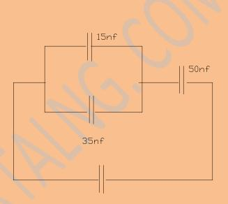
i. Capacitance of parallel circuit is  $C_T = C_I + C_2 = 15\mu f + 35\mu f = 50\mu f$
