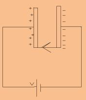
An Insulator called a dielectric may be placed in the space between the plates in close contact with them.
